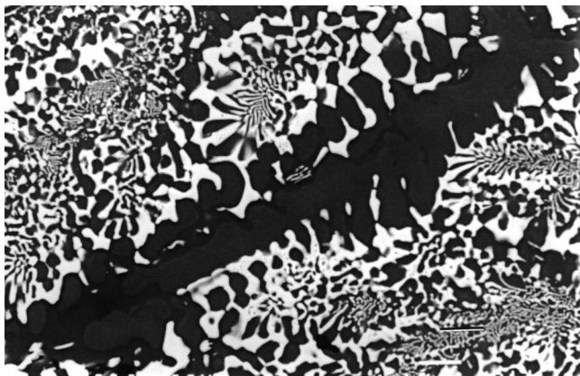
Fig. 1. SEM image in backscattered electron mode: Nominal \text{Al}_{64}\text{:Cr}_{21}\text{:Ni}_{15} (ANC019) showing \text{Al}_9\text{Cr}_4 dendrites (medium grey), \phi peritectic layer (dark grey), with \text{Al}_9\text{Cr}_4 + \text{Al}_3\text{Ni}_2 (light) eutectic. Bar represents 10 \mu\text{m} .
